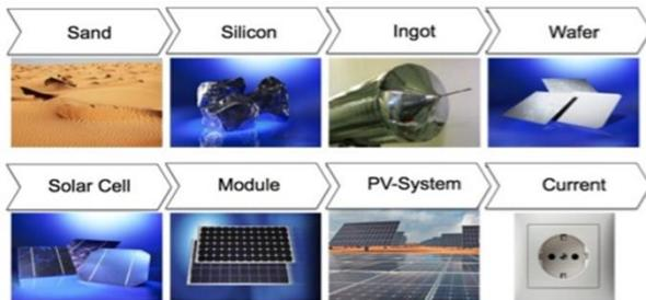
Fig. 4. The main manufacturing steps of solar cells.
