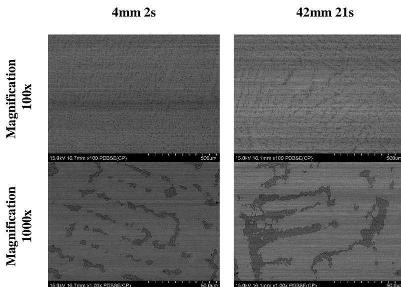
Fig. 8. SEM observation ure of the selected cast samples: (  $d = 4$  mm  $t = 2$  s), and (  $d = 42$  mm  $t = 21$  s).
