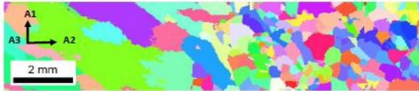
Fig.6. A3-IPF EBSD maps of the Cu-Mg alloy rod for the pull distance  $d$  and the  $d= 36$  mm  $t = 18$  s (A2 represents the continuous casting direction).
