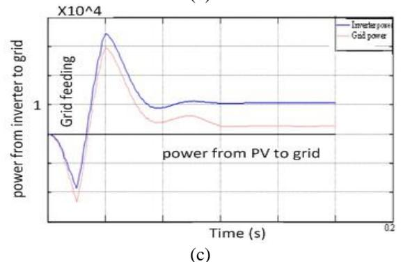
Fig. 5. (a) Load demand power, (b) Inverter output power, (c) Output power from the inverter to grid
