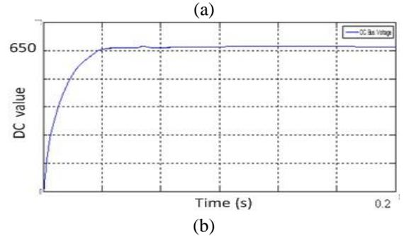
Fig. 4. (a) Output power under irradiance level  $900\text{W/m}^2$ , (b) DC bus voltage
