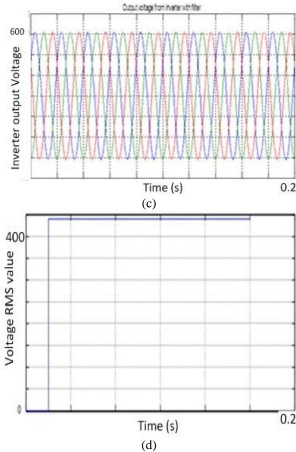
Fig. 9. (a) Effect of using filter on DC bus voltage, (b) 3Q voltage from inverter without filter, (c) 3Q voltage from inverter when using filter, (d) Voltage RMS value.
