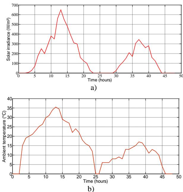
Fig.12. a) Solar irradiation and, b) temperature profiles
