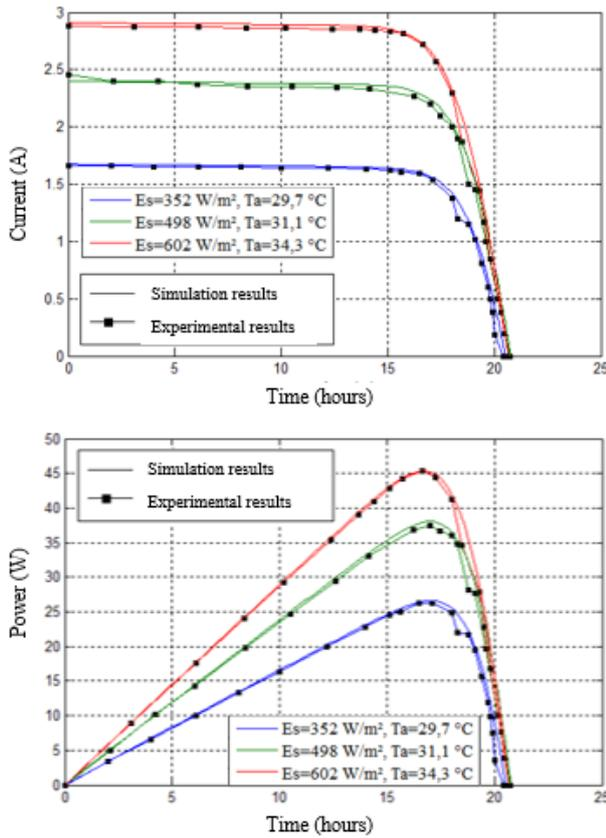
Fig. 4. Obtained I-V, P-V curve simulations and experimental results
