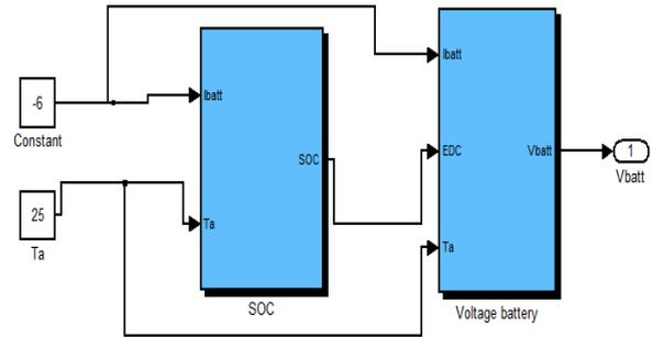
Fig. 6. Battery model used in MATLAB/Simulink
