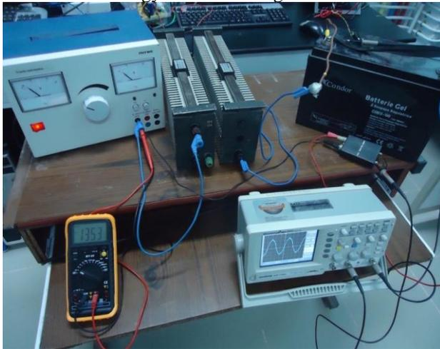
Fig.5.Used lead acid battery and test setup
