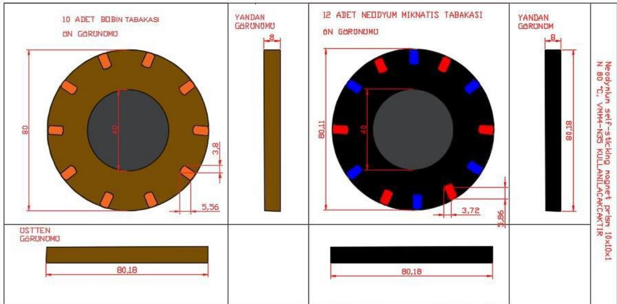
Fig. 4. The winding diagram and the position of the magnets on the rotor disk.
