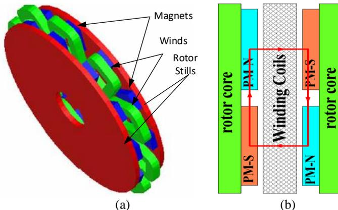
Fig. 3. Coreless EASM model (a), Cross section and distribution of magnetic field (b) [12, 19].
