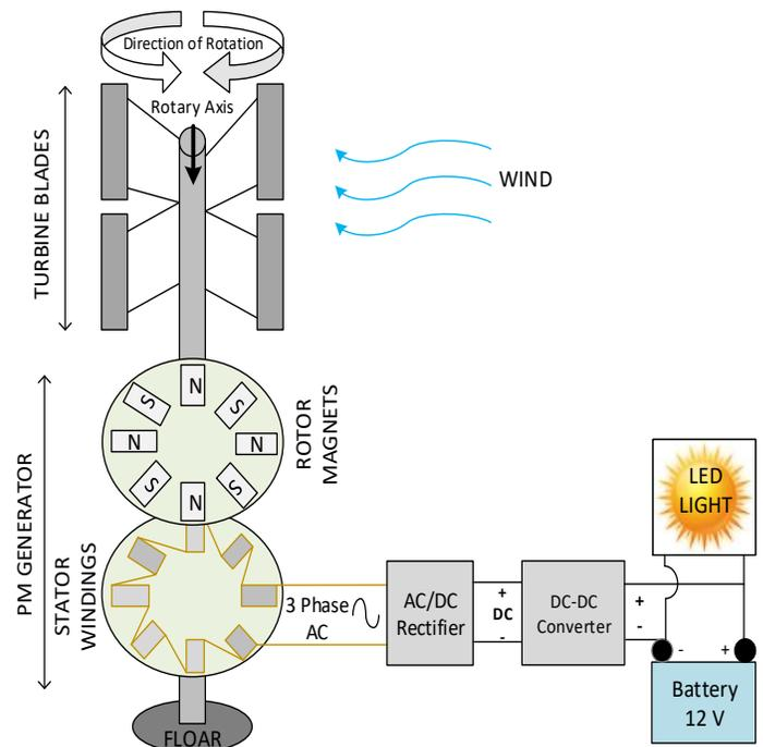
Fig. 1. The general structure of the vertical axis wind turbine and its components.
