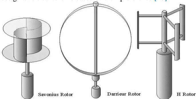
Fig. 2. Three types of vertical axis wind turbine models [18].
