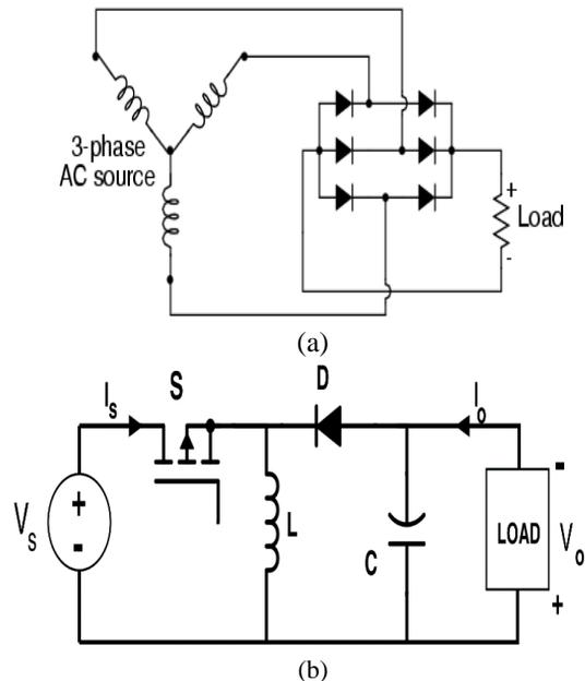
Fig. 6. (a) Three-phase rectifier circuit, (b) The DC-DC buck-boost converter.
