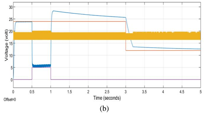
Fig. 12. The simulation results for the short circuit inrush conditions. (a) Buck mode for 12 V input and open circuit during the 3 to 3.5 second, (b) Boost mode for 12 V input and short circuit during the 0.5 to 1 second.
