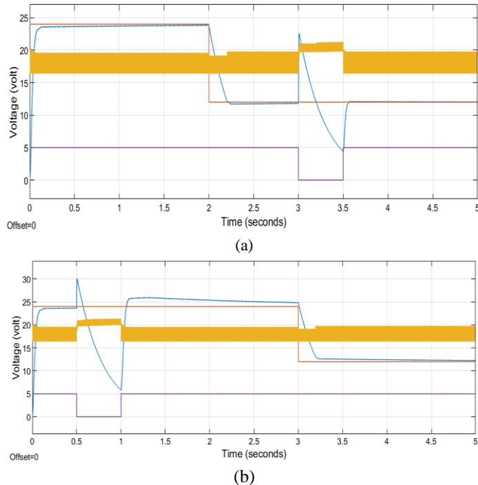
Fig. 11. The simulation results for the open circuit inrush conditions. (a) Buck mode for 12 V input and open circuit during the 3 to 3.5 second, (b) Boost mode for 12 V input and open circuit during the 0.5 to 1 second.
