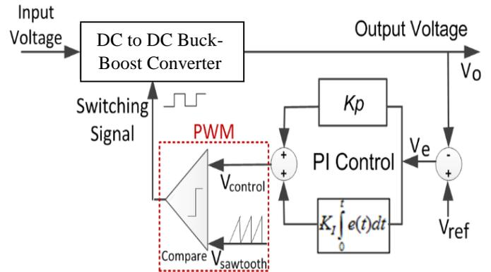
Fig. 7. Block diagram of the DC-DC converter with a PI controller [23].
