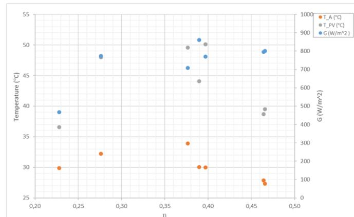
Fig. 5. Temperature correlations for amorphous silicon PV module.
