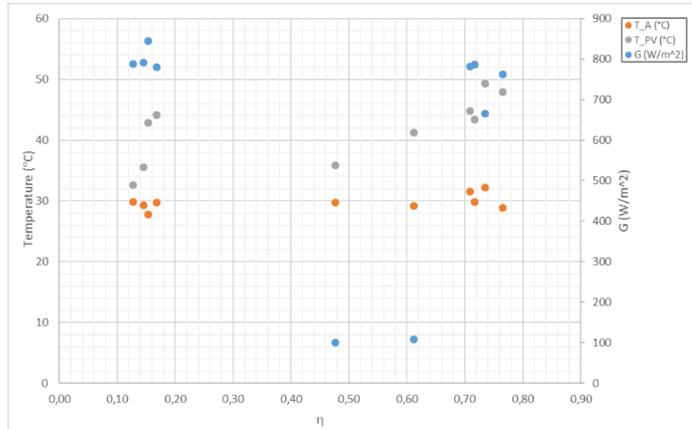
Fig. 4. Temperature correlations for monocrystalline PV module.
