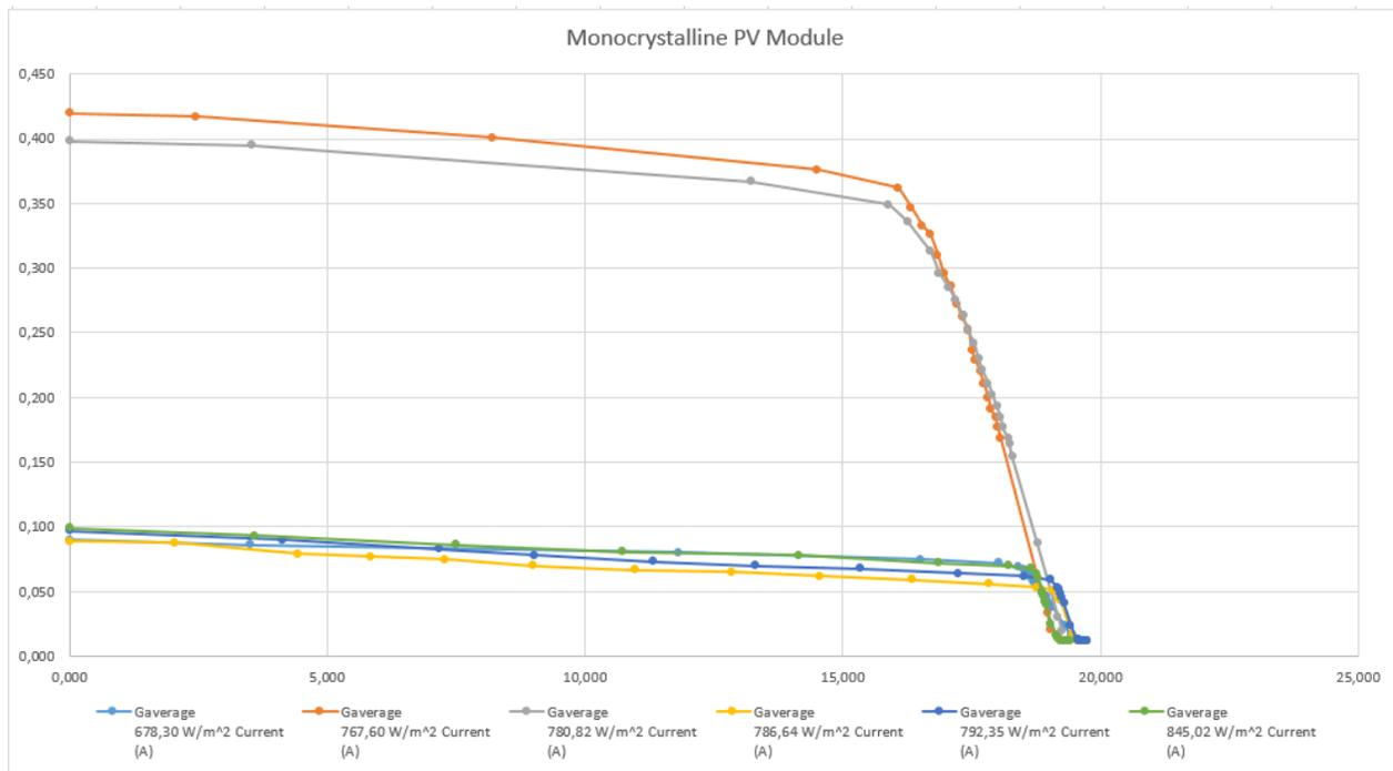
Fig. 3. I-V Characteristics of Monocrystalline PV module.
