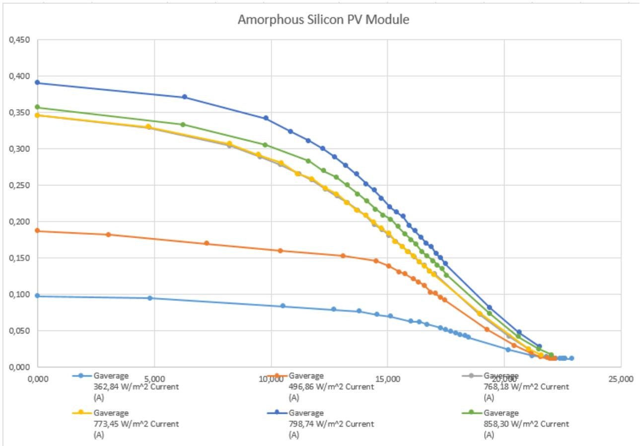
Fig. 2. I-V Characteristics of Amorphous Silicon PV Module.
