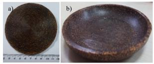
Fig. 2. Waste bio-composite applications a) teapot base b) tea plate.
