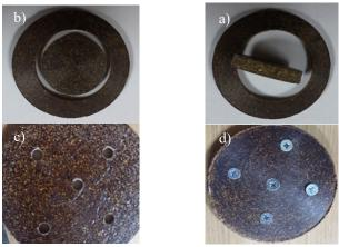
Fig. 1. Machinability properties of produced composite material a-b) punching process c) drilling process d) screwed joint process
